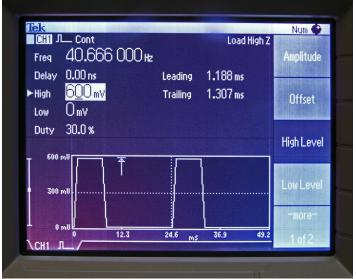
Here you can see that the frequency is set to 40.666 Hertz. That corresponds to a rotor RPM of exactly 610. I can also shape the pulses to look just like the output of the Hall Effect sensor.
