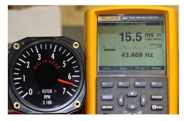
Lastly I decided to check the accuracy of the indicator. It was way off but there is an adjustment in the back. I calibrated it over the range from 600 to 650 RPM. With the mill indicating 650 RPM, 43.469 Hz on the Fluke 287 translates to an actual RPM of 652.04. I'm shooting from slightly below to avoid a reflection so the parallax error would make the indicator look slightly low. Bottom line – it's now close enough. December 19, 2009
