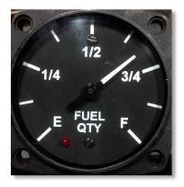
And here's the UMA fuel quantity indicator indicating2/3 full. Once I have a working fuel system I'll measure the output of each probe as fuel is added in carefully measured increments. When I have that data I can tweak the code to account for the irregular shape and exact capacity of each tank. When I get to that part of the project the ability of the Arduino board to do complex math will make the choice of a digital approach obvious.
