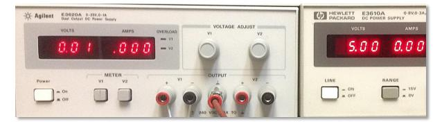
Here's my test setup – The left power supply represents the upper tank and its set to 0.0 volts which represents an empty tank. The right power supply is set to 5.00 volts, or a full tank.
