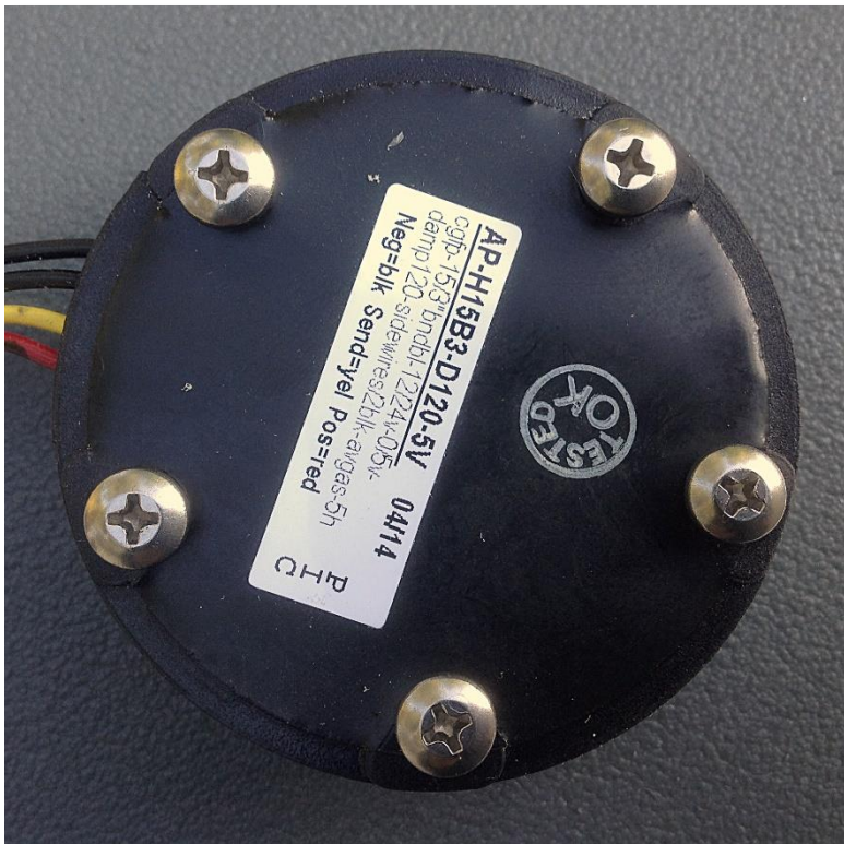
Figure 10 – The next step, which is even easier, is to install the top O-ring and then the fuel probe with the O-ring sealing screws.
