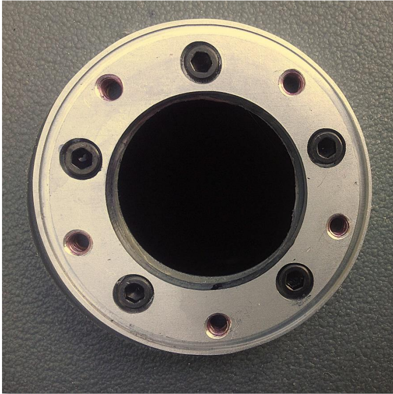
Figure 9 – Here's the plate mounted on my top tank. It was a very simple process to install the bottom O-ring on the mounting plate and then hold the nut plate inside the tank with one finger while lining up the mounting plate and getting one screw to engage. Once one screw is installed the others are installed as you see. The socket head cap screw heads are all recessed below the surface.
