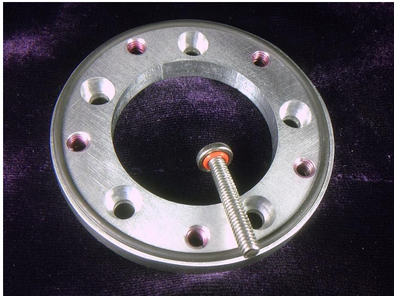
Figure 6 - Completed Fuel Probe Mounting Plate
