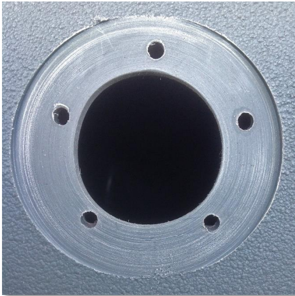
Figure 8- Prepared Fuel Probe Mounting Hole
