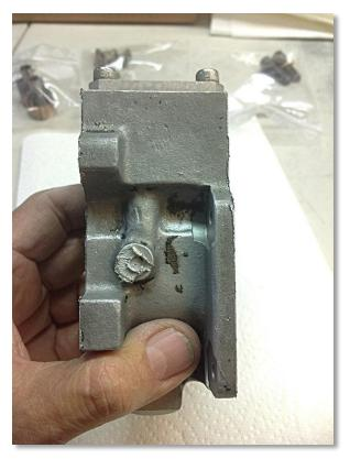
Here's the pump housing after blasting it with fine ground glass. The few remaining flecks of paint are solidly bonded to the aluminum.
