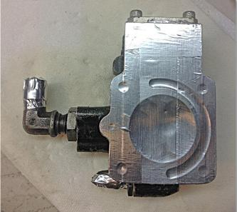
Here's the pump ready to blast. I used fine ground glass and I was extremely careful to seal every opening. After blasting I inspected the pump with a magnifier and cleaned out any specs I found with a Q-tip and alcohol.
