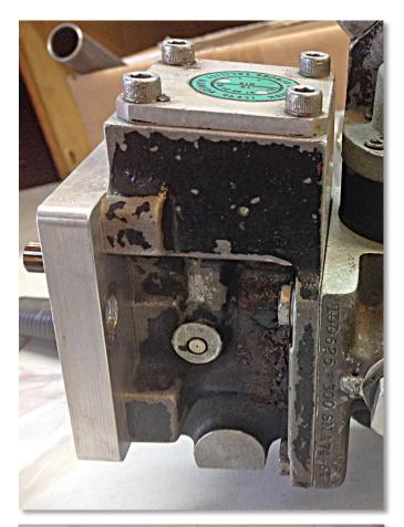
I started with the fuel pump assembly which I removed and tore down. I pulled the mounting pad and filter cover off and polished those parts. I also replaced the hardware.
