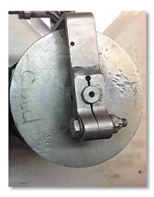
The bottom of the torque motor has a small crack and what looks like many hammer marks over the crack. There isn't much I can do about that.
