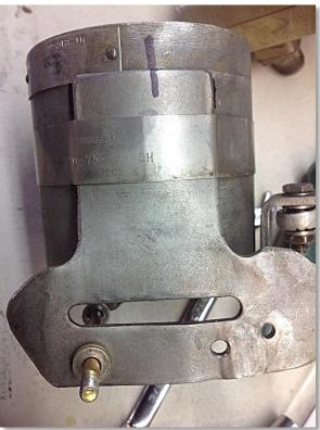
The torque motor had seen some hard times and this mounting plate looked like it had been fabricated out of some scrap. The slot and the ears served no purpose at all, so I cut the ears off and went after the plate with my deburring wheel and polisher. It's stainless and polished up nicely. I also polished the clamp which was also stainless.
