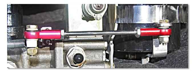
I replaced the old stiff Heim joints with new anodized aluminum ones and also adjusted the torque motor lever's height on the splined shaft so that the rod ran parallel to the direction of motion.
