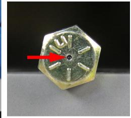
27 March 2011 -- While I was waiting for the finishing and blending putty to dry I checked in with my Guru, Hap Miller. He suggested drilling a very small center hole on the bolt that goes on top of the rotor head. During checkout the lead/lag adjustment process involves running a line from the tip of the master blade to the tip of the slave blade and adjusting the lead/lag of the slave blade to place the line directly
