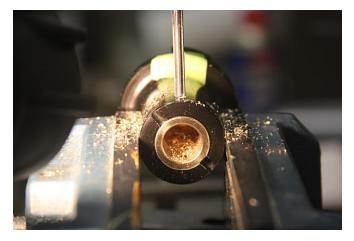
Now that the first hole is finished I checked it by tapping an AN bolt into position. Next I sawed off the head, cut the shank to the length I wanted, and deburred the ends.
