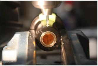
I used a series of three progressively larger drills and then finished off each hole with a precision reamer. Here's the first drill about to start on the far side of hole number one.
