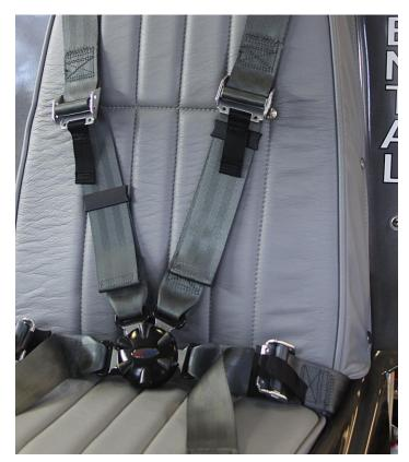
My harness is now installed. It's a TSO'd product from Amsafe. This configuration for the Helicycle has its own part number now so anyone wanting one like this can order by that number and not have to go through the process of determining all the critical lengths like I did.
