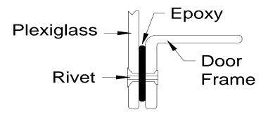
I want to paint the door frame with Zolatone and I'm not sure how the paint shop will deal with this. The epoxy bond is uneven. Sometimes it's down inside as I show here, and sometimes it squished up and over the top of the door frame slightly. On the outside the exterior paint needs to come up even or slightly above the door frame to hide the epoxy and the rivet heads. I should mention that I also smoothed out the
