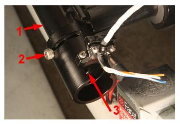
The throttle pot assembly is installed. To secure it I'll drill and tap a mounting hole through the collective shaft and into the large anodized piece at #1. It has to be a short screw so it doesn't interfere with the rotation of the internal tube.
