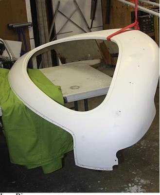
I've always had trouble finding a stable way to hold the cabin halves while I work on them. I finally came up with this approach. I place the flat area formed by the windshield across the table top and suspend the lower part of the cabin from the rafters using this old nylon tie down strap. The strap is tied at the center of balance and the old green sheet under the other side keeps the cabin from sliding around on the slick surface of the table and also protects it from damage.
