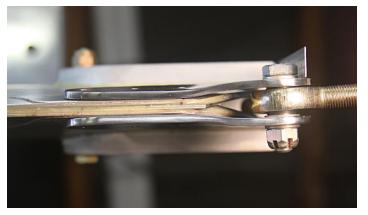
Here's a side view showing the twists and bends in these brackets as well as all of the layers of doublers and skin that make up the main rotor blades.
