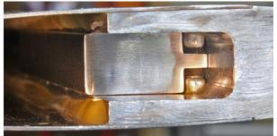
Here's the blade tip with the outer two rivets nicely nestled in their milled slots, and the weight flush against the forward edge of the extrusion.
