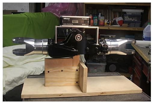
I painted the end plugs last night and while I wait for the paint to dry I made this stand to hold my rotor hub for static balancing. I added a saddle that spans the center of the hub so I can sit my protractor on it and measure the angle of the hub. I machined the two legs at the same time so they're the same exact length. In this picture the left side is down by 0.01 degrees.
