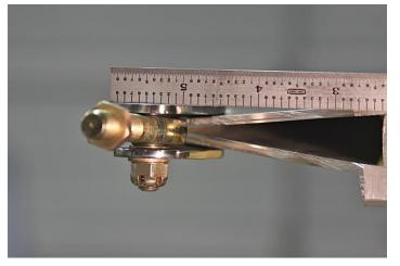
Here's a look at a bracket pair mounted to the drag link end bearing. You can see that the surfaces that will mount to the blade are not parallel. I need to spread this pair apart but also get the twist just right as well. This is going to be tricky, but it's the first step before even thinking about drilling those holes. I also want to strip off the paint and get down to bare metal.
