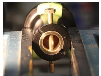
I used the pin I made from the bolt to hold the two pieces in alignment while I repeated the process with the second hole. I started again by lining up the chuck on the next hole to drill using another of my modified bolts as a guide.
