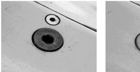
I've also been machining my replacement stainless steel tip weight screws to get them flush with the skin. On the left is a stock screw, and the right is the screw after machining and polishing. Once the balance is complete my plan is to fill in the gaps and the Allen head with finishing and blending putty, but if I use my gloss black 3M tape to make stripes on the tip, or clear 3M tape for the leading edge, I may not need to bother since the screws would be covered over with the tape.
