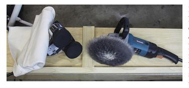
Here are the two types of buffers I'm using. I have separate compounding pads for each grade of polish for the circular buffer. The random orbit polisher uses that fleece on the left. You have to find a clean area and then hold the fleece by wrapping the excess around the handles. You can keep moving around to about six different spots before the fleece is ready for the washer.
