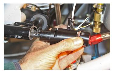
Here's the business end of the throttle tube with the tube sticking out of the collective. The largest piece I'm holding has a clearance hole for that tube so it slides through and into the back which is hollow. That piece pushes into the collective tube all the way until it bottoms out. If you lined the hole up correctly it will line up exactly with the slot above my thumb.
