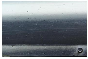
16 January – Two more weeks have passed and I'm still polishing the same side of the same main rotor blade. I've spent an entire weekend working on the outer two feet on one side. My blades are in terrible shape. In this picture you can see many very small pits. They're proving to be extremely difficult to polish out because they're quite deep. These pits are unsightly and can serve as the starting point for corrosion.
