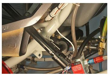
And here it is with the collective all the way up. I want to make sure that there is a nice service loop on the pot wire so it doesn't get snagged or abraded on anything, or stressed during operation. With the strain relief in place all the flexing takes place along the length of the wire and it's not concentrated at the weakest point – the solder connections.
