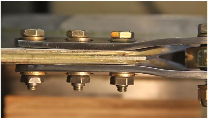
Here's the finished assembly after flipping the blade over and countersink the bottom bracket. The end bearing bolt doesn't need to be countersunk because of the twists in the brackets.
