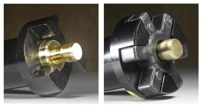
With the rear of the brass insert flush with the back surface of the coupling, the spider fits on perfectly. Now comes the hard part – match-drilling the two holes so the bolts will pass through the drive shaft tube, the coupling, and the insert, and still be a press-fit all the way through.
