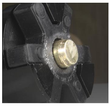
With the spider in place you can see that the flat portion of that brass center piece is mostly buried inside the spider. In fact the only part of the brass piece that was engaging the gear box shaft was the chamfered portion, and the inside of the gearbox shaft is also chamfered so it was engaging chamfer-to-chamfer, which is to say, really not at all.
