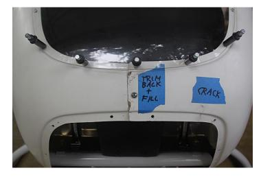
20 March – Now that the main rotor blades are static balanced the only thing left to do is finish off the cabin. Before I can have the cabin painted I need to patch a few dings, pits, voids and cracks. The most visible are here in the very front between the chin window and the windshield.
