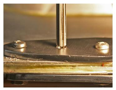
Then I finished off the hole with a precision reamer. I know everything is perfectly lined up and the hole is plumb because of the previous steps I've taken. I haven't shown it because my lubricant is a foam and covers everything up, but I used a lubricant when cutting.
