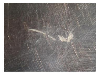
I decided to change projects and start polishing the tip end of this blade. This picture shows an area about 2-inches by 3-inches with some nasty scratches or pits that you can easily feel with your finger nail. Since it's near the tip the surface is critical and I want to smooth these out. I started with 600-grit wet and dry sandpaper and then switched to 1000-grit. After a few minutes of light sanding in this immediate area I switched to Nuvine G6 course grade polish.
