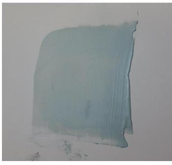
In this picture I've applied a thin layer of the Evercoat blending putty to an area that had several small scratches. I could have smoothed out that area on the right a bit so I would have less work to do later, but this is fine.
