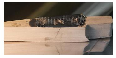
While I'm focused on the blade tips I decided to epoxy a small piece of screen over the holes in the end plugs to keep wasps from making a nest inside my blades. Centrifugal force will keep the tip end plug screen from pulling loose since it will be pressed up against the wood in flight.
