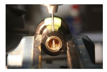
I've slowly enlarged the hole using the three drills and now the reamer is about to finish off the first hole.
