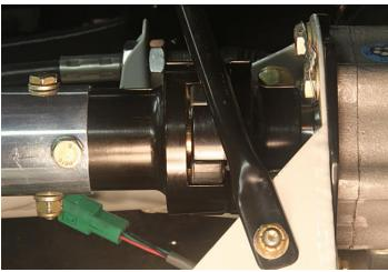
After lubricating the interface with grease I reinstalled the coupling onto the tail rotor drive shaft. That's the end of that project until the factory mechanic/test pilot comes out and aligns the driveshaft using a dial micrometer jig.
