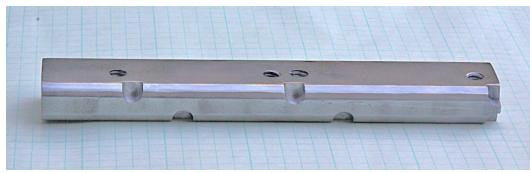
22 January – I machined my tip weights yesterday. I started by chamfering the forward side to match the shape of the leading edge extrusion. This
