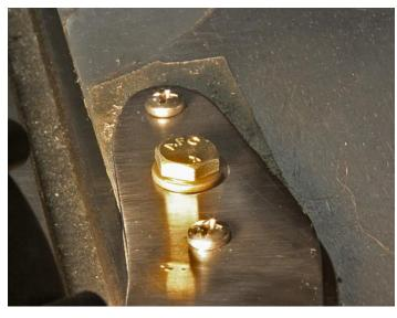
After using AutoCAD to confirm that I could safely countersink these spots I used a 0.500 end mill and ran it down exactly 0.054 inches as my drawing called for. Here's the result.
