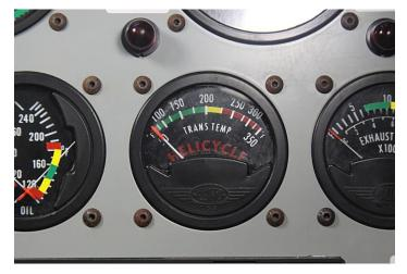
30 January 2011 – In the space of one year all the black button head cap screws I installed on my instrument panel have rusted, simply sitting in my garage. I don't live is an especially damp climate and nothing else in the garage is rusting like these screws.
