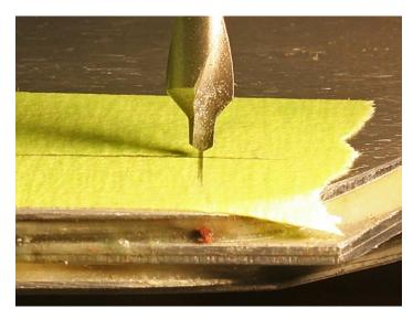
It's finally time to drill into my rotor blade. I think I have a workable plan. First I marked out the location of the first mounting hole from the dimensions on the plans. Then I center drilled the hole.
