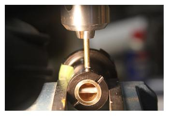
Now the brass insert is in position and I can center drill the starting point of the first hole so it lines up exactly with the existing hole in the coupling. I want to remove material from the brass insert but not the coupling – easier said than done!
