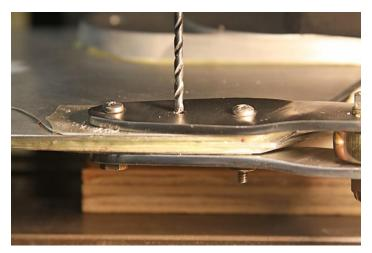
I secured that spot with a 6-32 screw and nut and moved to the other end of the bracket and repeated the process. I've got the long axis of the blade lined up with the mill base so all I had to do was move in one axis to get from hole to hole.
