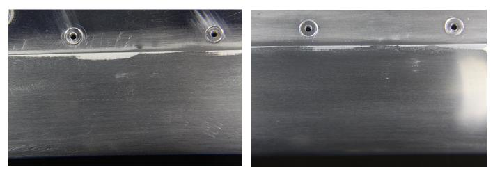
The picture on the left shows the surface after sanding with 400 grit and the picture on the right is the same general area after finishing with 1000 grit. The difference appears subtle but the final surface is satin smooth and ready for polishing. It took about 4 hours to finish the leading edge of one blade on one side. Its filthy work and disposable rubber gloves are handy.
