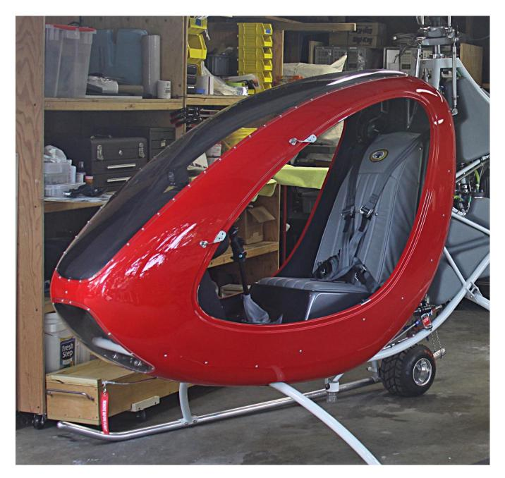
Here's a side view, and a shot of the left rear on the next page. I've left the throttle pot wiring disconnected until checkout, per instructions. Next to the right skid you can see my blade box, and that's my pitot tube under the belly, with the red 'remove before flight' banner.
