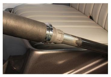
Here's the grip partially slid into position on the collective shaft. You can see how the fingers will grip the shaft when the knurled piece is tightened since the inside is cone-shaped. I had to sand the paint off the shaft to keep the friction down to a manageable amount. When the grip is in position the fingers are rubbing on paint.
