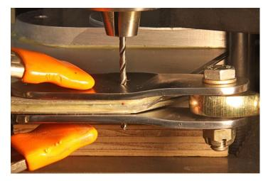
Without moving the bed I switched to a clearance sized drill and lined up the two brackets. They're bolted together using the end bearing to get the alignment top-to-bottom, and the spacing. I stuck them down using thin double-backed tape and held them in position with a clamp. Once I'd drilled through the rotor blade, and knew the hole on the bottom bracket was lined up correctly, I enlarged the hole to take a 6-32 screw.
