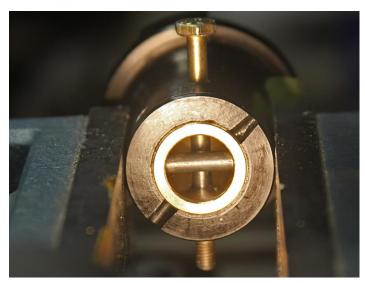
After repeating the process on the second hole I checked the alignment and fit by tapping another bolt into position.
