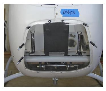
The area between the lower fuel tanks and the rear of the cabin is very cramped. In flight everything in this area moves except the fuel lines. I don't want those fuel lines to rub against the swash plate control tubes that run up from the mixer. I need a new plan...
