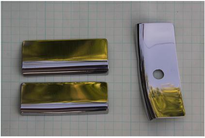
02 October 2010 - I've mounted the three striker plates on the left door lip, and I've learned a few things... 1) If you're going to do this, do it BEFORE you drill the mating holes for the door latches because the thickness of the plates moves the door just enough to throw your hole alignment off. 2) Don't bother polishing the plates until you're completely finished because they'll be all scratched up by the time you get everything fitted.
