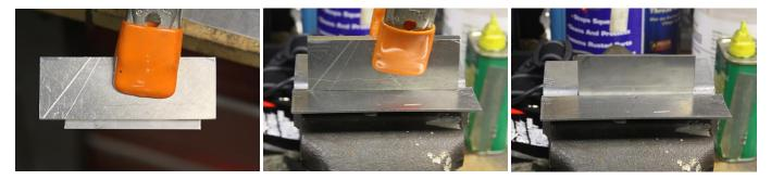
I used a scrap of <sup>1</sup>/<sub>4</sub>" stock to act as a guide, dropped it into my vise, clamped it down, and removed the guide.
