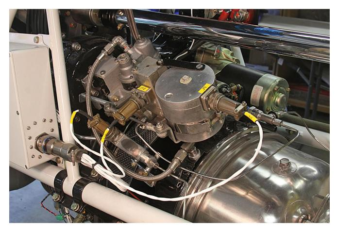
This is the final configuration with the new connectors installed. It's much better than my previous efforts. I would have preferred a right-angle connector for P9 to the throttle actuator but they're very expensive and no one stocks them. I plan to safety wire all of the circular mil connectors using .031 brass wire.
