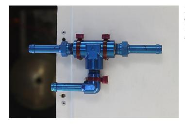
Here's the 'T' assembly mounted to the bottom of the right hand cabin half with three tie wraps. I made sure I didn't block one of the screws that attach the two halves.
