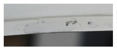
Here's what those voids look like after applying resin mixed with microspheres. I made a sandwich of a piece of Mylar and a wooden tongue depressor and clamped it over the voids to hold the resin in place and give me a smooth surface. The resin won't stick to the Mylar and the resulting surface is very smooth.
