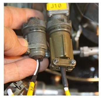
The connectors I have installed now (left) don't have any strain relief for the cable. Continued flexing during flight could cause a conductor to eventually fail. I'm switching to the version on the right. This backshell includes a strain relief clamp that captures the cable and produces a much more secure installation.
