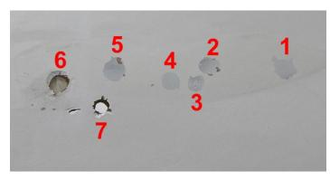
The auxiliary tank installation affects the alignment of the seat pan, and the seat pan alignment affects the cabin halves. That's caused me to have to move a few holes. When I took a close look at this particular hole I realized that the previous builder(s) had already drilled and filled 6 holes. My poor cabin looks like a piece of Swiss cheese. For the record, I inherited number 6 and filled it in and moved to hole #7!
