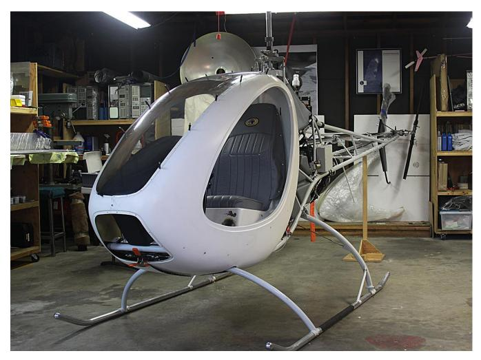
I'm moving on to the fiberglass now. I've secured the cabin halves to the seat pan using nut plates, and I have the wind screen attached using Cleco clamps. I'm a long way from painting the seat pan and the cabin but here's a partial list of work remaining before I think about painting the seat pan:
