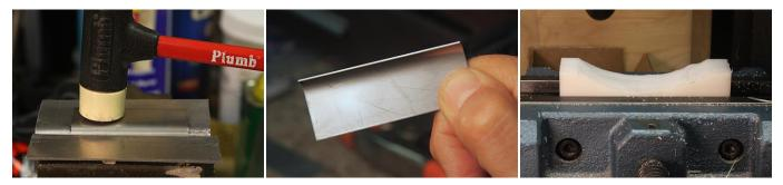
Then I used the guide to roll the piece over the jaw protector and finished it off with a few taps of my hard rubber hammer. That left me with the lip you see in the center picture. Next I made myself a form by tracing the curve on the door onto a piece of Delrin I had in my junk box. I milled out the general shape and then cleaned it up using a half-round hand file.
