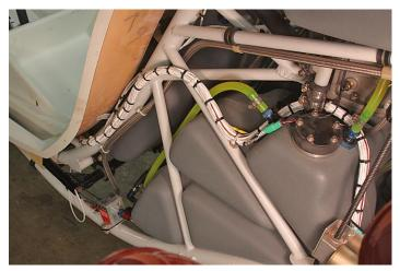
Oops! I thought I'd finally finished with wiring and I began to get the aux fuel tank ready to mount to the back of the seat pan. That's when I realized that the left hand cable harness interfered with the auxiliary tank. I had to disconnect the harness, pull it completely loose, and then reroute it around the outside of the frame tube. I also had to relocate the braided fuel line for the same reason. The aux tank is jammed between the frame tubes and there is zero room.
