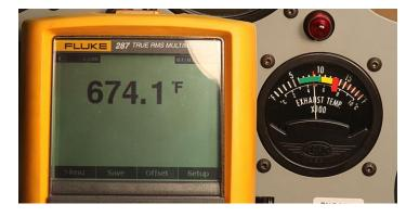
I temporarily hooked the ship's thermocouple to the EGT indicator using aircraft wiring. Then I attached my Fluke thermocouple to the ship's thermocouple and heated them both up with a temperature-controlled soldering iron that was cranked all the way up to 850°F. The temp stabilized as you see here. The EGT indicator appears to be reading about 200°F high. That's unacceptable.
