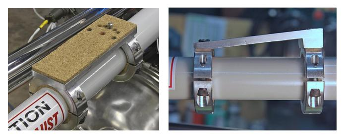
I can place these mounts anywhere I want on the frame tubes to get shots of the belts, cabling, the drive shaft, and so forth. I'd call all of those engineering test flight video.
