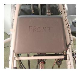
05 September 2010 – The auxiliary fuel tank is now connected. It will be clamped to the back of the seat pan. The next step will be to fill up the tanks and check for leaks. I should use kerosene or jet fuel but I have nowhere to store it once I'm done. I could leave it in the tanks but it's not a great idea to let fuel sit for many months, and if I have a leak I'll need to drain it out and put it somewhere, so I'll use gasoline for this test. I can use gasoline in my vehicles when I'm done.
