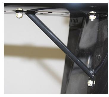
Here's the top vertical support detail, labeled #3 on the previous page. Care has to be taken here to make sure the tubing is clear of the tail rotor driveshaft coupling. That's why the bottom end is mounted to the outside of that triangular plate.
