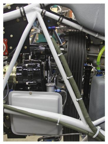
I'm jumping from project to project... Clickbond adhesive comes is a small foil dual-pack that contains enough adhesive for about eight to ten tie mounts if you work really fast. The adhesive has a working life of about five minutes or less. After deciding to put that one mount on the throttle actuator I needed to find a good use for the remaining adhesive. I decided to install a few more tie mounts to the right hand frame tube that the harness follows to access the battery box.
