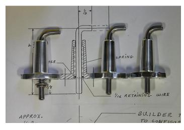
Here's an example of typical kit parts that need finishing. They're part of the door latch assembly. They come from the factory as you see on the left. I milled off most of the excess material using my mill (middle), and then used my disk sander to rough out the final shape, and finally I finish it off using my deburring wheel and then the polishing wheel (right.)
