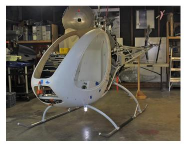
I managed to catch a shot of the lower strobe firing. The pattern is two blinks of the top strobe, then two blinks of the lower strobe. The pattern repeats about once every five seconds, and any time either main strobe fires the tail strobe also fires. It should help me be seen during daylight hours. I'm not planning on any night flights and the ship's exterior lighting does not meet FAA requirements for night flight.
