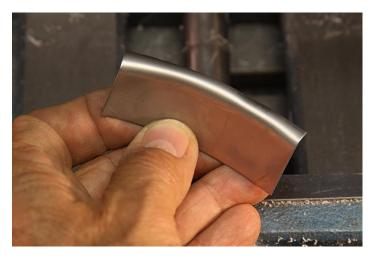
Here's the roughly formed part. It still needs to be deburred and tidied up and then polished. And of course the hole will need to be drilled in the correct location. I'll also drill two holes on either side for rivets.
