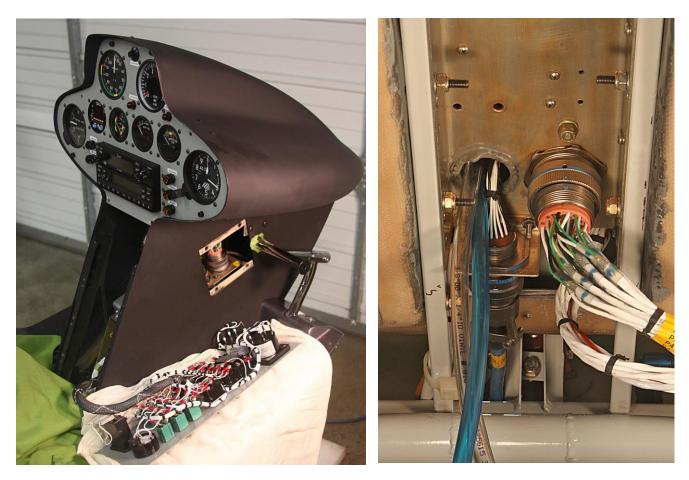
Left – The lower panel goes in last because it overlaps the top panel. This panel is a lot less work to install because there's only one cable.
