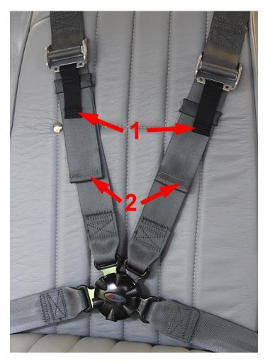
Here's a look at the Amsafe restraint system. I like the rotary buckle because you can easily get out of the harness with one hand. This is important because you might only have one hand that still works after a crash. You just twist the knob and all the straps pop loose except the one that you've designated as the fixed side. I made the right side fixed to keep the buckle from interfering with the collective.
