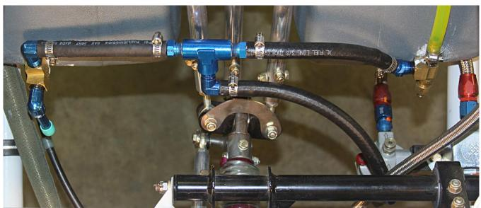
Here's the final configuration. The 'T' is about three-quarters of an inch in front of the tubes, and that's about where it will end up when it's tie-wrapped to the cabin. The remaining hose fitting on the left of the picture connects to the auxiliary tank.
