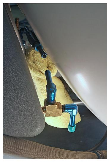
The right side is much simpler. The right side of the 'T' connects to the right-angle hose fitting. I'm going to rotate the brass fitting slightly from the vertical to point the hose fitting up towards the 'T' and also rotate the fitting slightly away from the tank and towards the back of the cabin.
