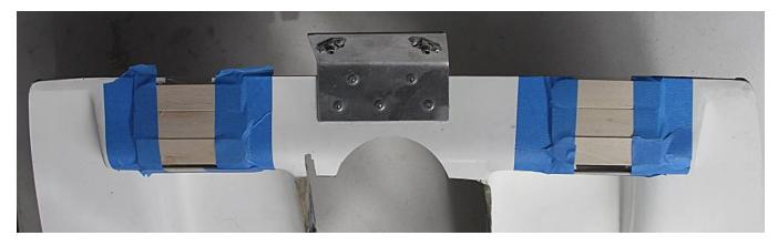
I've formed molds on the top side using tongue depressors over Mylar sheets. I was going to use thin aluminum sheets over the Mylar but I couldn't get the sheet to conform to the curve.
