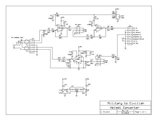
Military helmets are fitted with microphones and earphones that are incompatible with civilian radios so they either need to be replaced or their inputs and outputs need to be converted. I pulled a schematic from another pilot's web and it looked well designed. I modified it slightly and decided to have some printed circuit boards made up and try it out.
