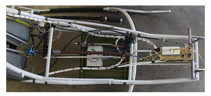
I've final installed the directional controls, the cyclic, the collective, and all of the cabling that will be covered by the seat pan. I'm now ready to finish off the final sanding of the seat pan and take it off to be painted. Once that's done I can install it and final install the instrument panel, the auxiliary tank, and the seat back.
