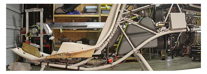
Here's the view from the left side of the ship. This view shows the completed wiring harness now attached to the frame with about fifteen Click Bond tie wrap mounts and several Adel and Nylon MS25281 clamps. I may go back and cover the harness with Nomex Roundit later.
