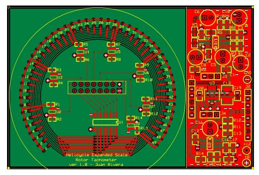
I completed the expanded-scale rotor tach LED PCB design and I had a bit of space left over on the right. I managed to cram all the components for the military-to-civilian converter board into the remaining space. With luck I'll have a helmet and a finished board to try in a few weeks...
