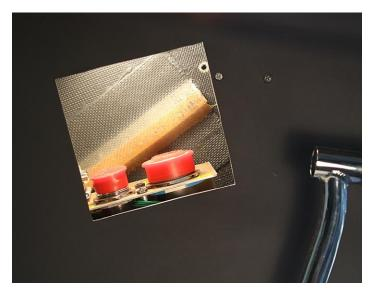
I'm adding an access panel to the right side of the instrument pod so I can get to the top instrument panel cable connectors where they connect to my interface chassis. I'll use Camlock fasteners to secure the cover. I've also drilled two small access holes on the other side of the seat pan to allow calibration of my altitude encoder.
