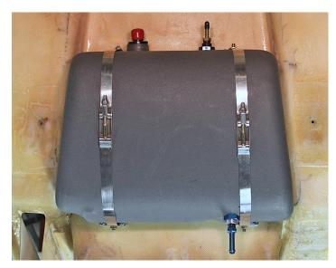
Here you see the auxiliary fuel tank temporarily mounted to the seat pan. Because of the taper it must be inserted from the bottom. It's a jam fit.
