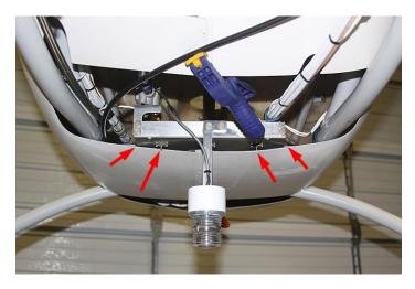
This is the view after trimming the bottom of both cabin halves and installing my lower strobe light. I'm still not comfortable with the clearance at the edges of the shelf (outer arrows), and two of the six screws I'm using to secure my strobe electronics are also in the way slightly. I think I'll remove those two. The four remaining screws are strong enough to lift the entire helicopter off the ground. That box isn't going anywhere, even with two screws removed.
