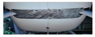
10 October 2010 – It's true. The last ten percent of the project takes ninety percent of the time. I've been working on the small details that I need to attend to before I can think about painting the cabin. I fabricated this forward gear cover plate from .031" 6061-T6 supplied for the purpose. Match-drilling and installing the eight nut plates into the fiberglass while
