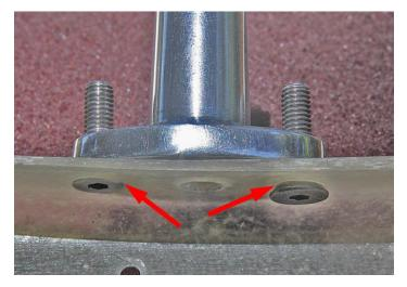
Before I can bond the Plexiglass to the fiberglass door frame I have to locate and drill all of the mounting and access holes for the three latches on the left hand door. (The right hand door is bolted in and has no latches.) I could do it after the Plexiglass is bonded but then I'd risk scratching it and have poorer access.
