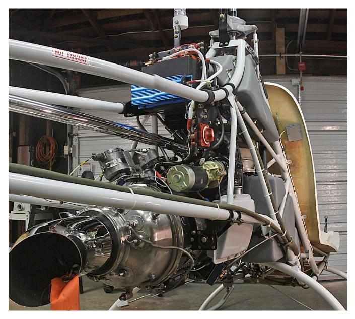
Here's a stitched picture of the right side of the ship. Since the main harness uses the bottom frame tube to access the area under the seat pan it bypasses the tight area around the auxiliary fuel tank, making this side much simpler. On this side I simply tied the harness to the frame using tie wraps and no Click Bond mounts. I might switch to the mounts once I'm satisfied with the routing.
