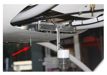
Other than paint, and installing the pitot tube and static port, the underside is almost complete. The red arrow points to the transponder antenna. The brass piece in the upper right is one of two fuel drains. Before a flight I can drain a sample of fuel to check for contamination from water or debris.
