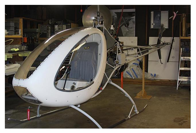
I applied the adhesive and riveted the Plexiglass to the fiberglass last night. This evening I ground the pop rivets flush with the inside of the door and popped it into place. The next step is to fabricate and install the door hinges and then trim the door frame. I found a few dulled-up areas where the two windows must have rubbed together during shipment. I'll have to polish those out.
