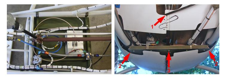
In my initial design of the tray that I've installed under the seat pan I didn't pay sufficient attention to the clearance inside the cabin. I ran into an interference problem at the back of the panel on both sides (#2 in picture at right.) I also have a problem with the direction control cable from the pedals to the tail rotor. I don't want to cut slots as I've sketched (# 1.) I'll attach the lower strobe light to the rear of the tray (# 3.)
