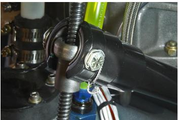
I purchased a 5-port manifold from Aircraft Spruce and connected all of the static lines. The input comes from the static port in the belly and the four outputs go to the altimeter, VSI, and air speed indicator, and to the encoding altimeter that feeds the transponder. The blue line will attach to the pitot probe and also goes to the air speed indicator. That instrument uses the difference between ambient static pressure and ram air pressure to determine air speed.
