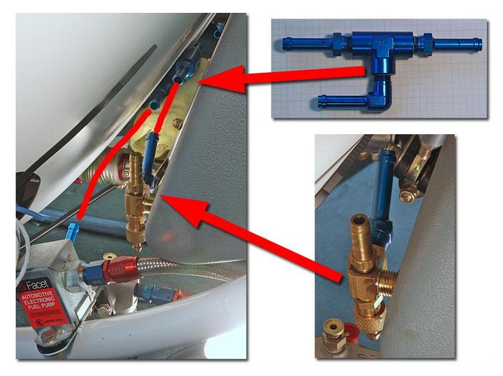
While I'm waiting for the remaining fabric I'm back to the fuel system. I've decided to mount the 'T' assembly (upper right) against the back of the cabin using tie-wraps. In the picture at the left it's held in position with a rag. One of the tubes I'm trying to avoid is just visible peaking out from the side of the tank. I should have good clearance between those tubes and the fuel lines connecting to the 'T'.
