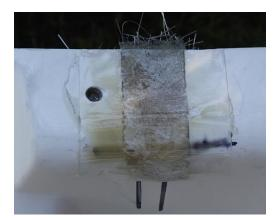
I laid up the fiberglass using a Tap Plastics polyester resin. The tongue depressor/Mylar backing conformed to the shape of the front surface as well as could be expected so a minimum amount of sanding should smooth it out. I'll add one more layer on the back side to increase the strength. Once I cut out the new slots I'll find out if the patches are strong enough. There shouldn't be much stress in this area so I hope it will be sufficient.
