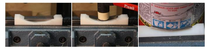
The next step was to place the flat piece in the form and gently tap away at it until it took the shape I wanted. Now comes the tricky part... As the piece takes the shape of the large radius it tends to straighten the lip. I found that I could clamp the piece against the form by squashing it against my largest fire extinguisher. Then I was able to go along the lip and tap it back into the shape I wanted.
