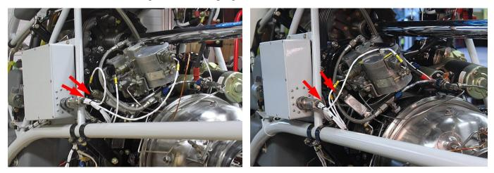
Here's the before and after views from left to right above. Now I have more clearance for the main fuel solenoid and the wiring is much more secure, but after thinking about this overnight I've decided to replace all three of these Cannon connectors with a type that has a strain relief backshell. The existing connectors don't adequately protect the individual wires from vibration.
