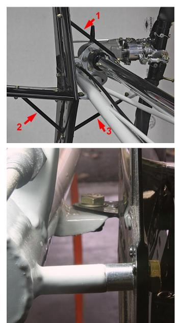
The tail fins are braced with three supports. The standard kit has you make these from chromoly steel tubing by squashing the ends in a vice, but I chose to have Hap Miller make me a set by welding flat mounting tabs to the tubing.
