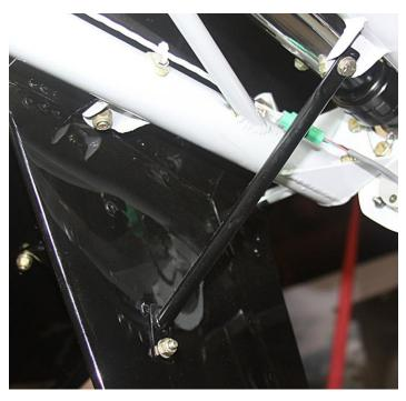
And here is a shot from below of the third support. That wraps up this project. If necessary the factory checkout pilot will be able to make tweaks to my alignment by changing the width of the spacer (vertical fin alignment) and ovaling out the bolt hole I just mentioned (horizontal fin angle of attack alignment.)
