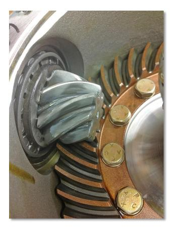
Here's a closer look at the pinion gear. When you consider that there is almost one hundred horsepower driving this little gear you can appreciate the engineering that went into the design of this transmission. As B.J mentions in one of his videos, the loads on a helicopter transmission are much more severe than on an automobile. I'm impressed!
