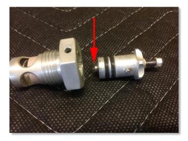
Here you see the removable piece with the magnet (red arrow) removed from the body. Notice that it is sealed with two O-rings. You can also see that the valve has now closed off the opening to prevent leakage.
