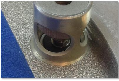
Here's the chip detector installed in the new enlarged hole. In this picture the transmission is right side up and you can see how the lubricant will be able to flow freely through the holes in the side of the detector. The magnet is just visible at the bottom of the detector.
