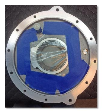
After tucking the transmission away I degreased the inside of the cover and sealed off all the sensitive areas to prevent contamination. Only the chip detector hole is exposed. Once I get going this side will face down so gravity should help me keep it clean.
