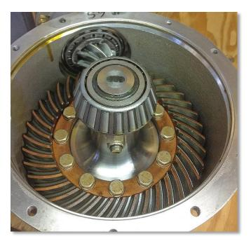
After removing the bolts and carefully working the bottom cover loose, I lifted it straight up and this is what I found. When Blake talks about preload he is talking about the tapered roller bearing at the top of the picture (bottom of the transmission.)
