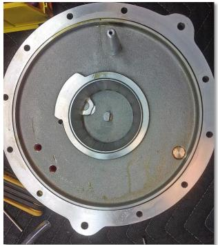
After carefully covering the transmission to keep it clean, I moved to the bottom cover. You can see the very thin O-ring that goes around the circumference. I removed that and set it aside in a baggie along with the plumbing and hardware.
