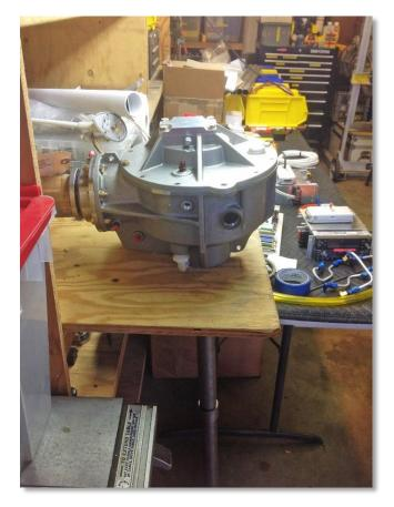
Here's the transmission supported by the shelf with the hole in the middle and ready for the operation to begin.
