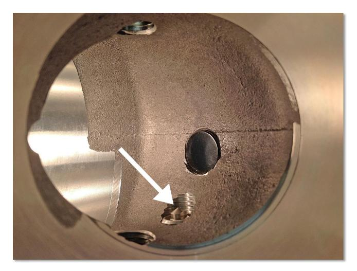
Here's a look inside the housing. As you can see, the chip detector is completely out of the way of the gears (while arrow) and in a great place to pick up any ferrous material in the oil. To insure that the interior of the housing was completely free of contamination I washed it out in the kitchen sink with a few drops of dish soap and lots of hot water. Once it was completely clean I dried it with high-pressure air and reassembled it.
