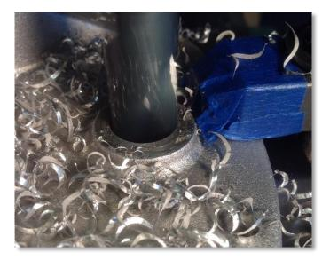
Once the hole was drilled and tapped I used this countersink to cut an O-ring groove. Again, this was made easy with a mill because I could take a .010 cut, pull the countersink out of the way, take a look, and then go back and remove a tad more material. The alignment remained locked in place during the whole operation.
