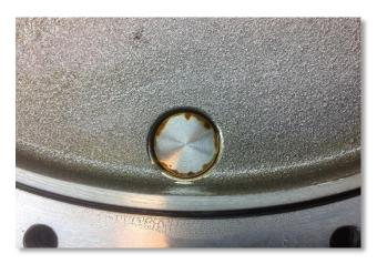
Here's a close-up of the existing chip detector hole. As you can see, there is almost no room to enlarge this hole without running into the outside raised area. When I'm faced with something like this I take measurements and draw it up in AutoCAD.
