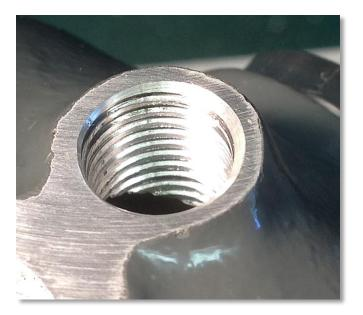
Here's the tapped and countersunk hole ready to accept the detector.
