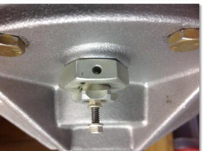
Here's what the sensor looks like mounted on the underside of the transmission. To check it all you have to do is grab the little ribbed piece, push up, and twist to remove. The signal line mounts to the threaded screw. This is one of the very few components that will use the frame as a ground return.
