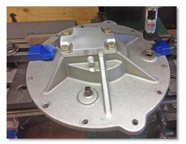
Here you can see the amount of offset that I used. Then I locked the bed down and used a variety of end mills and drill bits in successively larger sizes until I got to my final drill size of 11/16 which is the recommended size for tapping aluminum.
