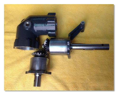
The tail rotor gearbox consists of two subassemblies that are inserted into precision honed pockets in the case. After removing the mounting hardware I was able to remove both after some gentle pulling and twisting, mostly required to break the paint loose where the parts joined. I set the parts on this new microfiber shop rag, took this picture, and immediately but them into sealed baggies.
