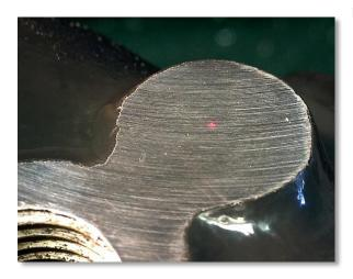
I surfaced the boss in preparation to drilling and tapping the mounting hole and used my laser center finder to eyeball the location of the hole (the small red dot.)
