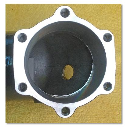
Here's the view of the gearbox interior looking in from one end. The hole that you see inside is the sight gauge.
