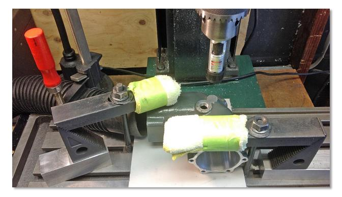
I clamped the housing in position being careful not to scrape up the paint. I also kept the clamping force to a minimum – just enough to secure the housing against movement. I don't want to distort it! Finally, I clamped my vacuum hose next to the opening on the left. My plan is to catch the debris that falls through the hole in the air stream before it has a chance to land inside the housing.
