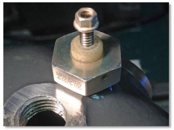
And here's the chip detector installed next to the drain plug.
