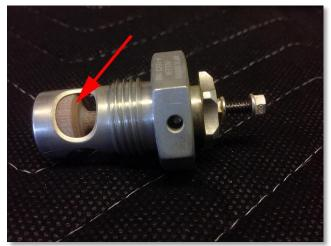
Here's a picture of the chip detector. It has two sections and is called "self-sealing." When the removable section with the magnet is removed the spring-loaded valve I'm pointing to will close off the opening to prevent oil from pouring out all over your fuel tanks.
