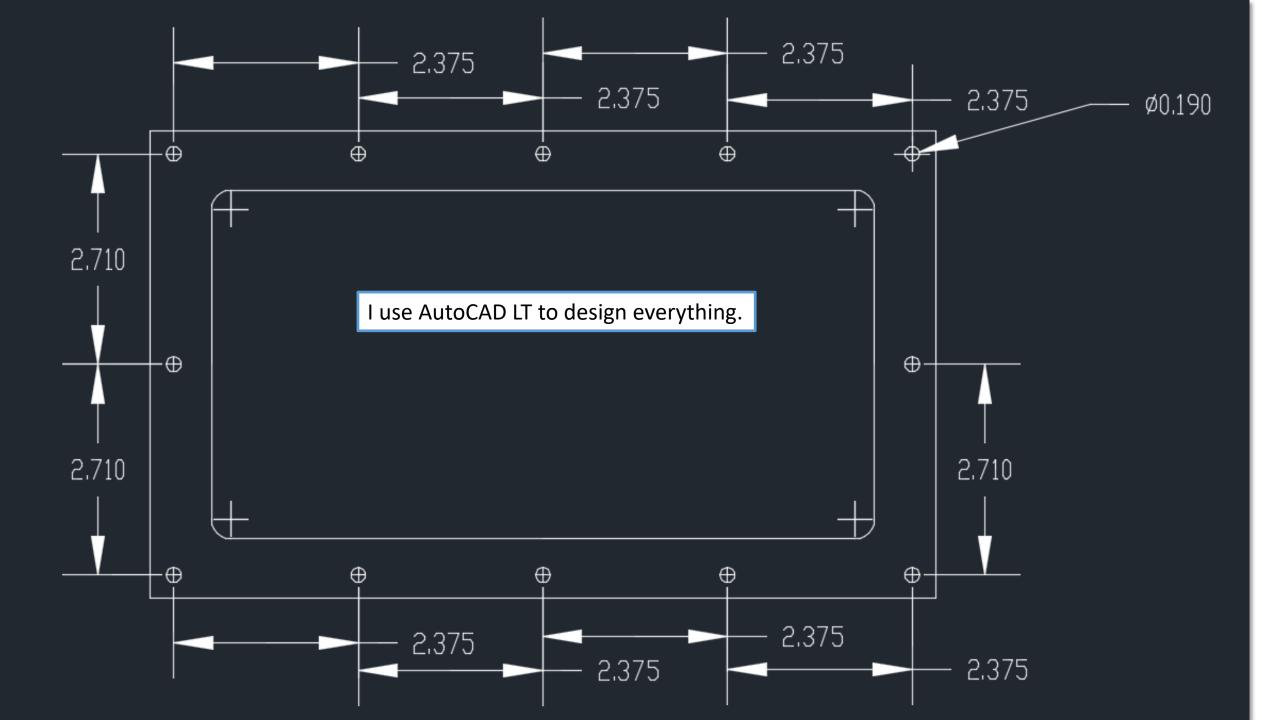
The gasket was made from a scrap of bathtub liner. I used 3M marine adhesive/sealant / fast cure 5200 on both sides of the gasket to seal the enclosure against water.
