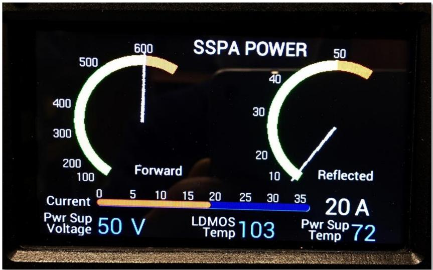
Set output power to 600 on Bird and HP meters, then adjust software scaling constand to make GUI meter read 600... I then lowered the power in 100 Watt steps and simply adjusted the X and X axis insertion points for the numbers.
