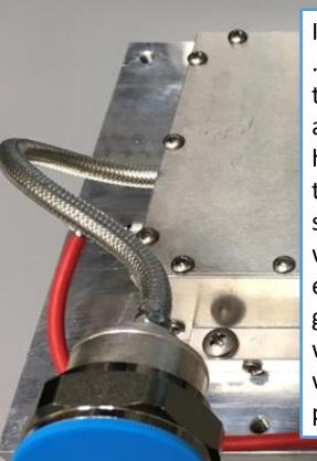
I fabricated this EMI enclosure out of .180 6061-T6 aluminum plate using a table saw with a carbide-tipped blade, and a milling machine. The pieces are held together with 4-40 screws, and the enclosure is secured to the heat sink with two rails that are attached with 10-32 screws. The base of the enclosure is lined with EMI mesh gasket material. The top and bottom were lapped using 400 and 600 grit wet and dry sandpaper to insure a perfectly smooth surface...
