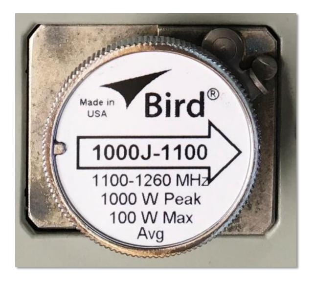
I'll use my trusty Bird Model 43 Thruline Wattmeter. I purchased this element especially for this project. It's only rated at 100-Watts average power because the center contacts cannot handle the high power and frequency and they will overheat.
