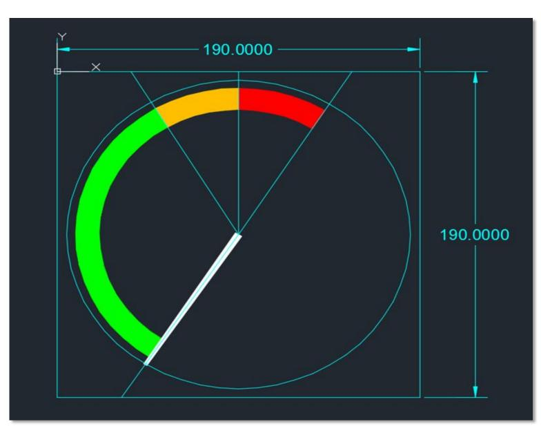
I called on my experience in aviation to model my meters after modern aircraft glass cockpit displays. I used AutoCAD for this first step. Each power meter will be 190 x 190 pixels in size.
