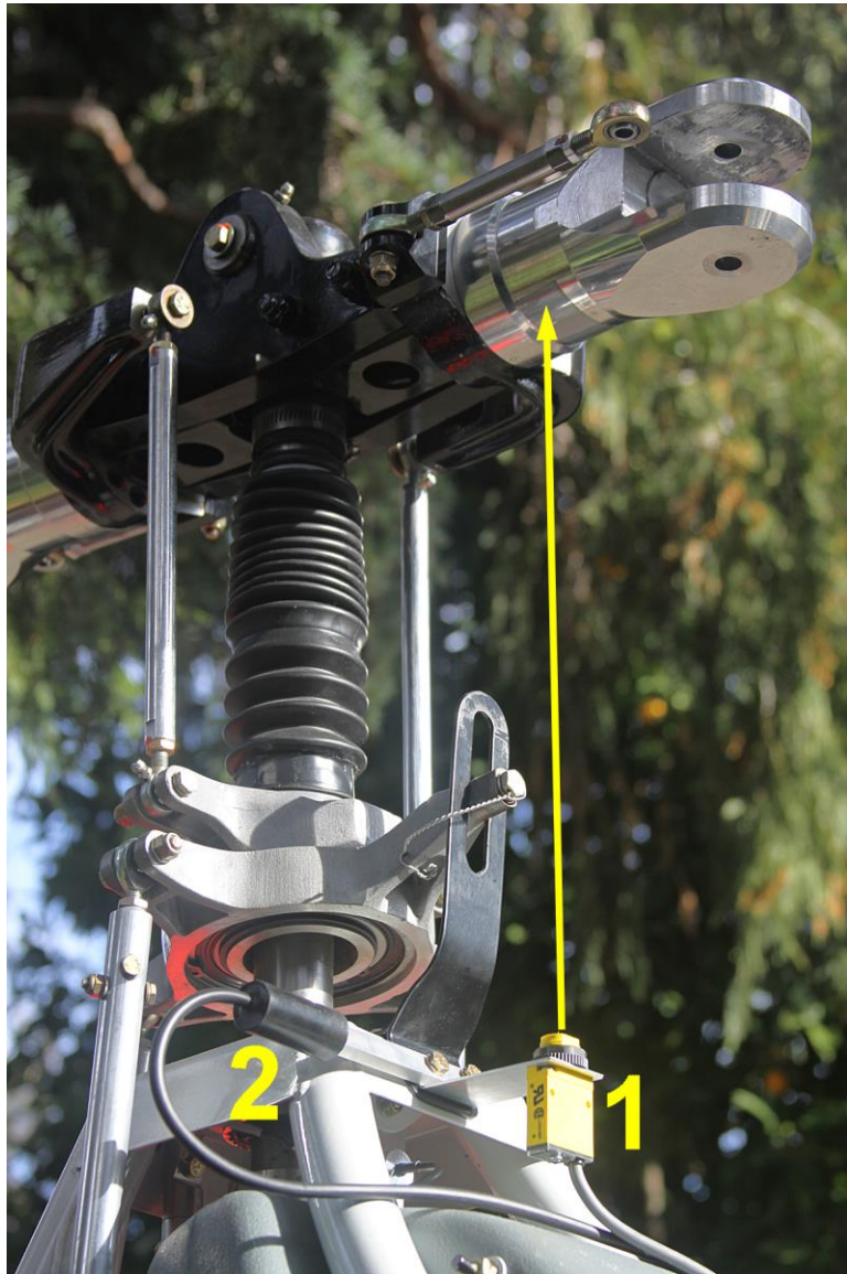
Figure 2— Vibration Analyzer Sensors
