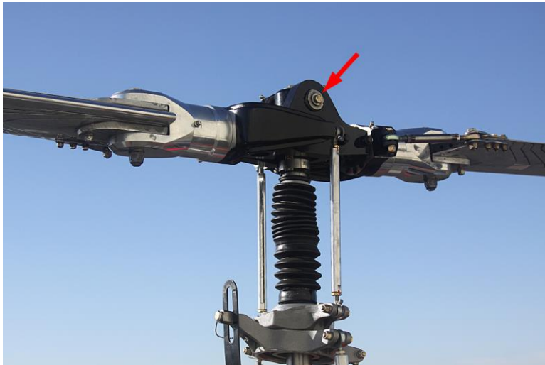
Figure 7 — Location of Rotor Hub Weights
