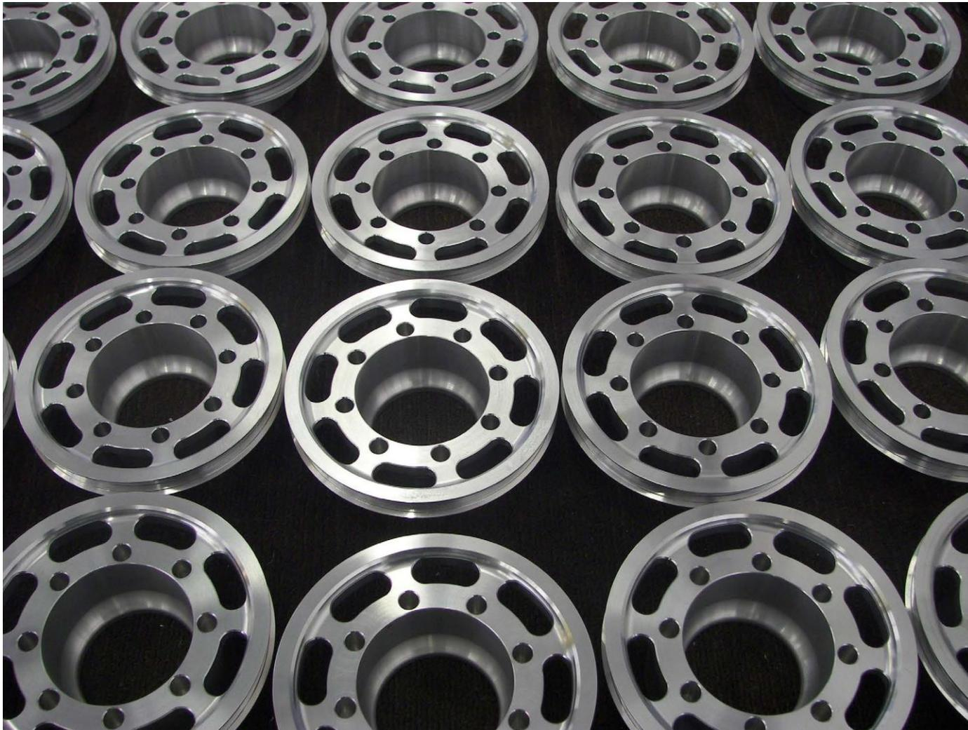
As of this week the pulleys have been machined and sent out for hard coating. This is a photograph of the aft side as it will be mounted to the transmission pulley.
