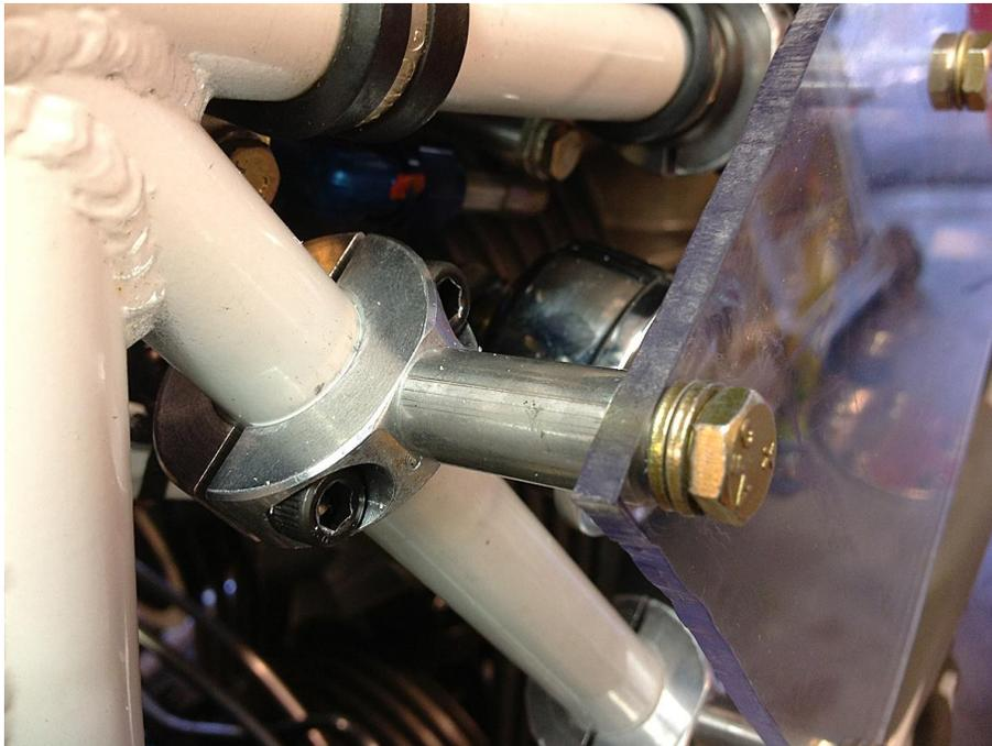
The mounting plate will be attached to the frame using four mounts – three of which form a triangle. The mounts consist of a modified two-piece shaft collar and a one-inch standoff. I machined a flat on each collar and tapped a 1/4-28 threaded hole to accept an AN aircraft bolt.
