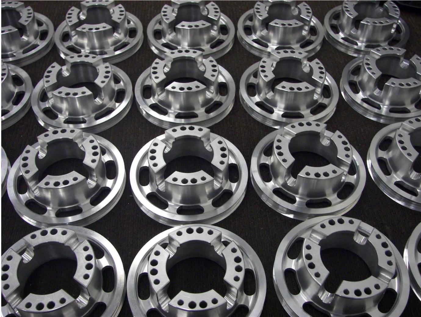
Here's a photograph of the pulleys viewed from the inside face that mates to the transmission pulley. Aren't they pretty? The eight slightly larger holes are for lightening and do not pass all the way through.
