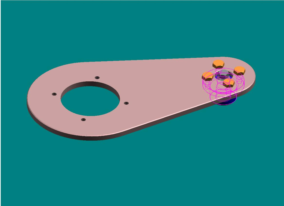
The spacer, with the alternator attached, mounts to this plate which mounts to the face of the drive pulley. This will perfectly align the two pulleys while the alternator mounting bracketry is being sorted out and installed. I'll certainly have much more on this once I have the spacer and the drive pulley in a week or two.
