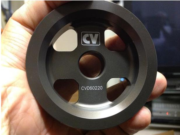
Here's the after market alternator pulley. It's also milled from aluminum and hard coated. It's a very nice looking piece.
