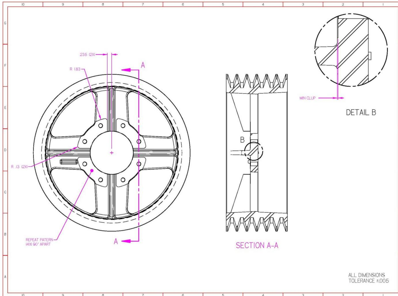
This drawing shows the cleanup area on the transmission pulley where the new drive pulley will mount. The fan ears must also be removed.
