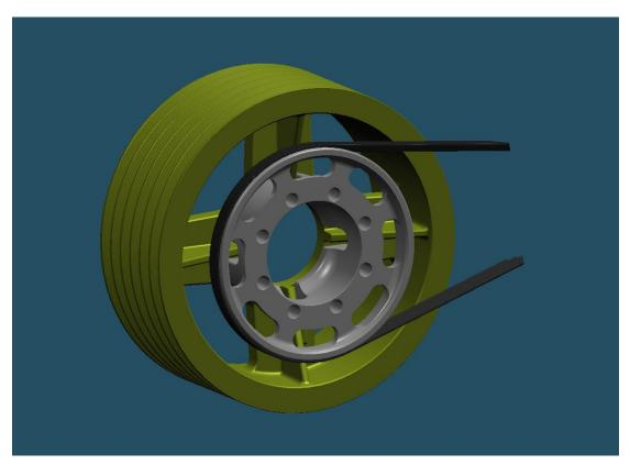
The drive pulley is CNC machined out of 6061 aluminum and hard coated for wear resistance. The alternator pulley is commercial off-the-shelf (COTS) from an automobile racing supplier. It is also milled from aluminum and hard coated
