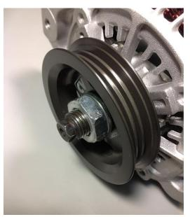
plane of the two pulley faces are exactly parallel, the alternator will be aligned in X and Y axis and forward/reverse direction and the belt will be in perfect alignment.
