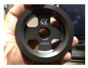
Here's the after market alternator pulley. It's also milled from aluminum and hard coated. It's a very nice looking piece.
