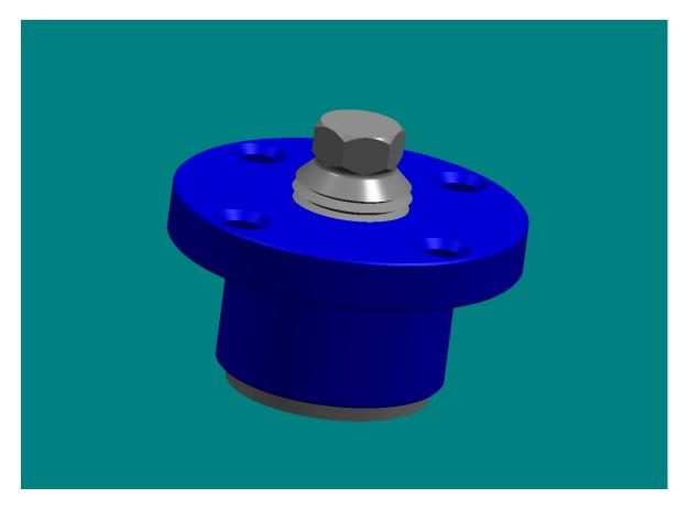
The alignment spacer, shown in blue, screws onto the existing alternator shaft shown in gray. The plate mounts to the face of this spacer.
