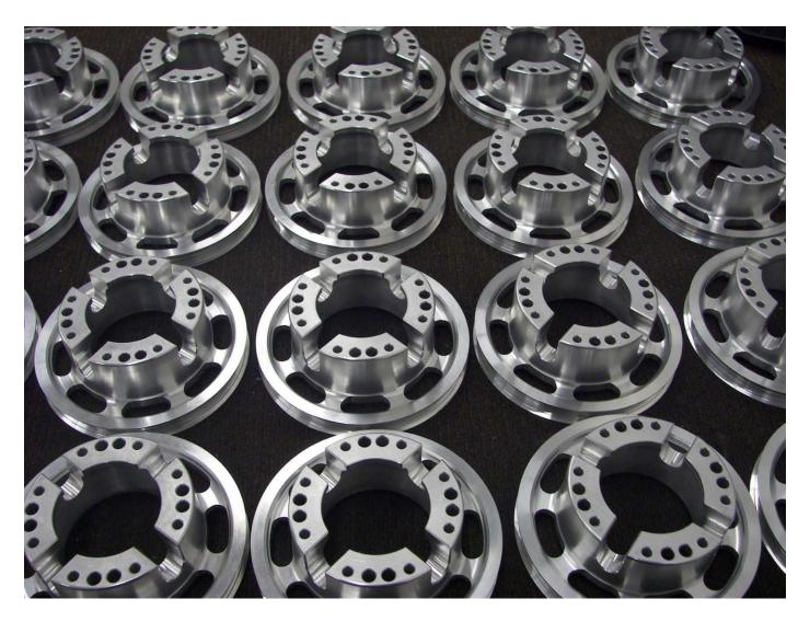
Here's a photograph of the pulleys viewed from the inside face that mates to the transmission pulley. Aren't they pretty? The eight slightly larger holes are for lightening and do not pass all the way through.
