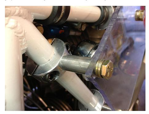
The mounting plate will be attached to the frame using four mounts – three of which form a triangle. The mounts consist of a modified twopiece shaft collar and a one-inch standoff. I machined a flat on each collar and tapped a 1/4-28 threaded hole to accept an AN aircraft bolt.
