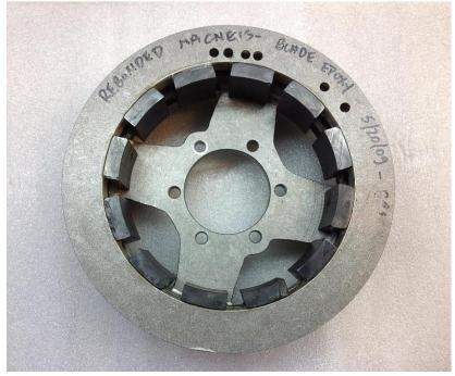
The existing factory charging system is designed around a riding lawnmower and is simplicity itself – there is a simple set of meager windings that are secured to the engine and a set of magnets that are epoxied inside the engine drive pulley. The factory "regulator" is really only a bridge rectifier that converts the pulsating AC output to DC. There is no voltage or current regulation and the current output is marginal.
