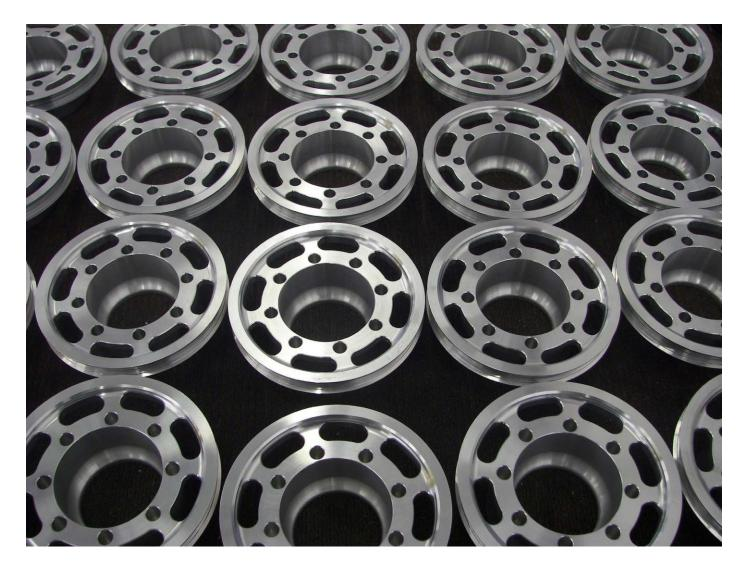
As of this week the pulleys have been machined and sent out for hard coating. This is a photograph of the aft side as it will be mounted to the transmission pulley.
